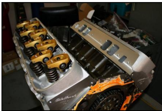
New Heads, Rockers and Pushrods Installed
