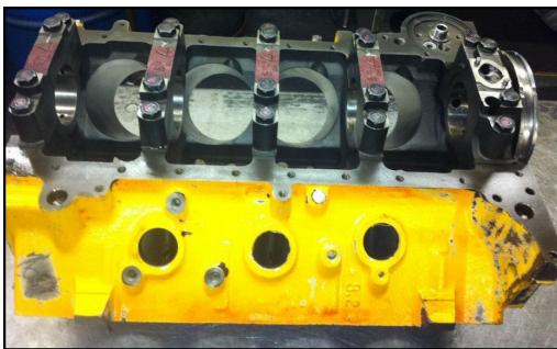
The motor after being media blasted
