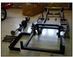
In spring thru the summer of 2016, we started with suspension, front and then rear end, and spring and 4 bars, 4 wheel disk brakes and routing of brake lines and the master cylinder. (It uses a smaller corvette master cylinder). The suspension height needed set up, so the wood wheels sized to the final wheel tire size were made. It looked funny, but worked well.
