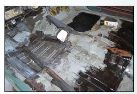
The interior was not ignored either. Bill stripped out the interior and found some holes in the floor board. He cut out the bad section, welded in a new piece and applied POR-15. Bill also installed new Pontiac seat covers, new door panels and carpet. The original steering wheel was cracked and broken, which Bill replaced with new and he also restored the steering column. Bill also bought new front and rear bumpers.
