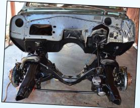
Bill started replacing the worn out suspension with an all new front end along with coil springs and shocks, all new brakes including a front disc conversion and added sway bars to give the LeMans a better ride. Bill also gave the rear end differential some attention and the steering box, which was replaced with new bearings and seals. Bill took a peek at the 326ci engine and found considerable sludge build up. He pulled the engine and sent it off for a rebuild.
