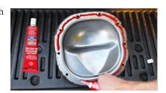
bottom of the trans. Then, you can thread the rest of the bolts in and snug them tight (not too tight as the gasket will push out).
