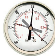
Poor Rings or Oil Open and close throttle rapidly needle pulls down to zero.
