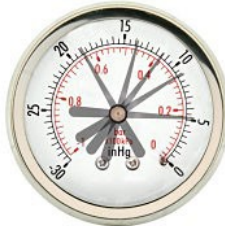
Leaky Head Gasket Between Cylinders Needle floats between 5 & 19
