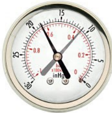
Burnt Valve Needle drops regularly several divisions
