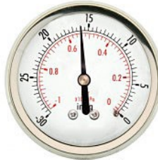
Late Ignition Timing Needle reads between 14 to 17 and remains steady
