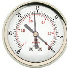
Chocked Muffler High reading at first, Breaks to 0 and builds back to 16
