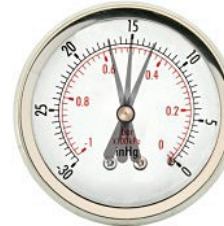
Carb Out of Adjustment Needle floats slowly between 13 and 17
