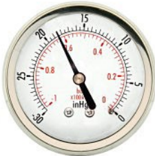
Normal Motor Needle steady between 17 & 21
