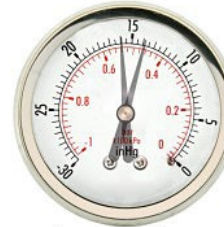
Plug Gap Too Close or Points not Synchronized Needle floats slowly between 14-17
