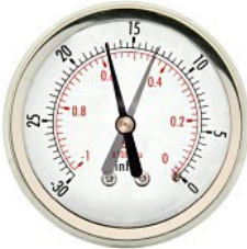
Sticky Valve Needle drops occasionally about 4 divisions
