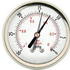
Leaky Valve Needle drops 2 or more divisions when valve should close
