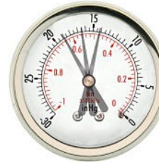
Loose Valve Guide Fast Vibration of needle between 14 and 19
